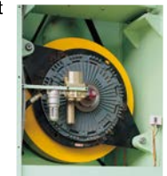
乾式煞車離合器 Compound clutch brake
